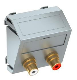
Multimedia support with two cinch connection sockets for audio R/L, slanting cable outlet, with labelling panel, two cinch couplings (RCA), socket-socket version, colour coding red/white. Support plate with locking fastening, suitable for horizontal and vertical installation in the system environment.
