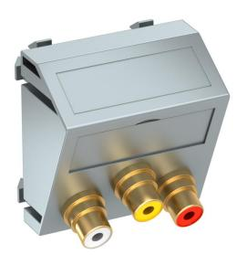
Multimedia support with three cinch connection sockets for audio/video, slanting cable outlet, with labelling panel, three cinch sockets (RCA) with soldered connection, colour coding yellow / red / white. Support plate with locking fastening, suitable for horizontal and vertical installation in the system environment.
