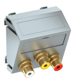
Multimedia support with three cinch connection sockets for audio/video, slanting cable outlet, with labelling panel, three cinch couplings (RCA), socket-socket version, colour coding yellow/red/white. Support plate with locking fastening, suitable for horizontal and vertical installation in the system environment.
