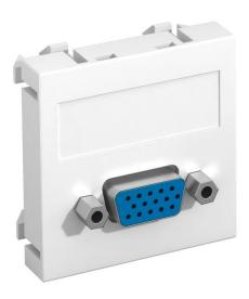
Multimedia support with one VGA connection socket, straight cable outlet, with labelling panel, VGA socket (HD15) with screw connection. Support plate with locking fastening, suitable for horizontal and vertical installation in the system environment.
