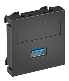
Multimedia support with one USB 3.0 connection socket, straight cable outlet, with labelling panel, USB 3.0 type A socket with screw connection. Support plate with locking fastening, suitable for horizontal and vertical installation in the system environment.
