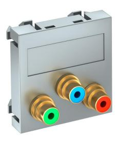
Multimedia support with three cinch connection sockets for component video, straight cable outlet, with labelling panel, three cinch sockets (RCA) with soldered connection, colour coding red / green / blue. Support plate with locking fastening, suitable for horizontal and vertical installation in the system environment.
