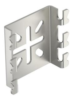
Mounting plate for screwless wall fastening of mesh cable trays. Accessories can be fastened to the mounting plate. In addition, the plate can be used for wall brackets.
