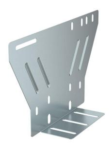
Universal mounting plate to fasten the FireBox T series to the rear side of cable trays and mesh cable trays as well as cable ladders of max. 60 mm side height. Enables the secure mounting of cables that maintain electrical functionality, without having to bend it over the side rail. Suitable for all FireBoxes.
