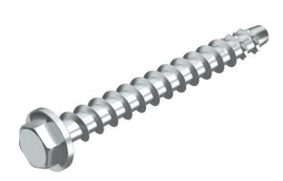
Bolt tie for direct mounting without additional anchors in cracked and uncracked concrete and masonry. With hex head drive and pressed washer to accept large loads. Suitable for fastening suspended loads from suspended supports and wall brackets.
