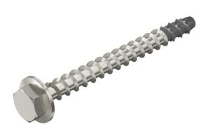
Stainless steel screw-in anchor for direct mounting without additional anchors in cracked and uncracked concrete and masonry. With hex head drive and pressed washer to accept large loads. Suitable for fastening suspended loads from suspended supports and wall brackets in wet rooms and in outdoor areas.
