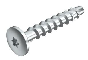
Bolt tie for direct mounting without additional anchors in cracked and uncracked concrete and masonry. With large round head to fasten mounting and profile rails. Torx drive T30.
