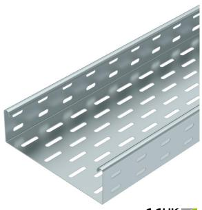
MKS 60 = Medium-duty cable tray system with a side height of 60 mm. The cable tray is fastened to the bracket with bolts, type FRS M6 x 12. The surface coating is a coating created in a single-dip method with extra-high zinc thicknesses
