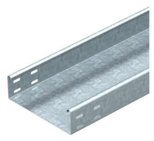
MKSU 60 = medium-duty cable tray system, unperforated, with a side height of 60 mm. Straight connectors should be ordered in the appropriate quantity. The cable tray has connector perforations on both sides.
