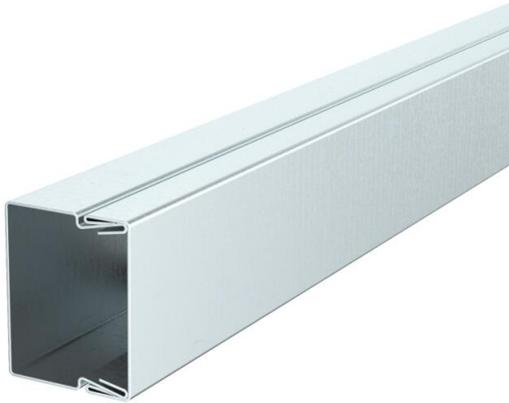
Duct cover and base with base perforation. Equipotential bonding is guaranteed between the cover and the base without any additional aids. The LKM cable duct, type LKM 20030, has been tested for the maintenance of electrical function as a routing system according to DIN 4102 Part 12. Please note the cable types tested in the BSS fire protection systems division!
