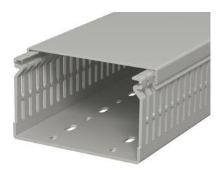
Wiring duct, incl. cover and base perforation, for horizontal and vertical routing of electrical cables in the switchgear cabinet. Designed as a metric duct. The nominal dimension of the system size corresponds to the internal dimension of the duct. Retainers are broken out without tools. The flush-floor routing of cables is possible through predetermined break points. Tapering in the side slots prevents the cables from falling out. Tested to DIN EN 50085-2-3. Special lengths on request.
