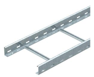
Cable ladder with perforated side rail of side height 60 mm with riveted C profile rungs, open in an upwards direction (NS version).
