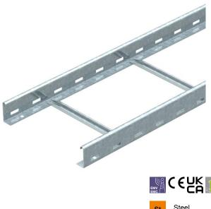
Cable ladder with perforated side rail of side height 60 mm with riveted C profile rungs, open in an upwards direction (NS version).
