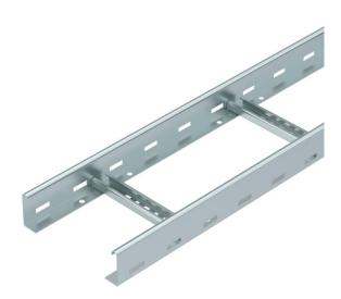
Cable ladder with perforated side rail of side height 60 mm with riveted C profile frames, open in an upwards direction (VS version). The cable ladder is shipped folded up.
