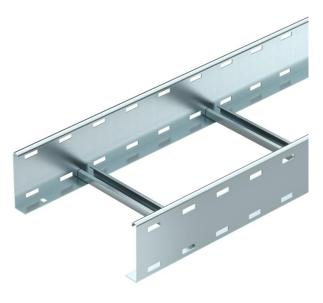
Cable ladder with perforated side rail of side height 110 mm with riveted C profile rungs, open in an upwards direction. The cable ladder is shipped folded up.
