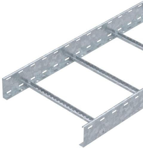
Cable ladder with perforated side rail of side height 110 mm with riveted C profile rungs, open in an upwards direction. The cable ladder is shipped folded up.
