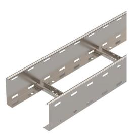
Cable ladder with perforated side rail of side height 110 mm with riveted C profile rungs, open in an upwards direction.
