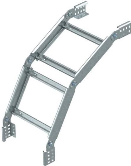
90° adjustable vertical bend, for cable ladders with medium-duty rung (VS) and a side height of 60 mm.
