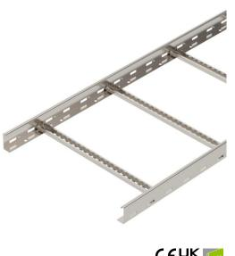
Cable ladder with 60 mm side height with welded C30 profile rungs which are open in an upwards direction. Rolled side rail for reinforcement and as edge protection. Fastening to the bracket takes place using clamps, type LKS 40. The slot dimension of the frame is 16.5 mm and the appropriate clamp clip is type 2056.
