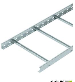
Cable ladder with a 60 mm side height with welded C30 profile rungs which are open in an upwards direction. Rolled side rail for reinforcement and as edge protection. Fastening to the bracket takes place using hold-down clamps, type LKS 40. The slot dimension of the rung is 16.5 mm and the appropriate clamp clip is type BS-H....
