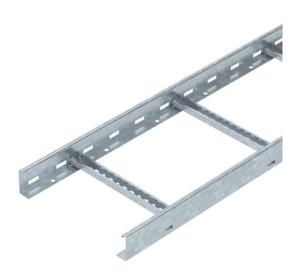
Cable ladder with a 60 mm side height with welded C30 profile rungs which are open in an upwards direction. Rolled side rail for reinforcement and as edge protection. Fastening to the bracket takes place using hold-down clamps, type LKS 40. The slot dimension of the rung is 16.5 mm and the appropriate clamp clip is type RS-H
