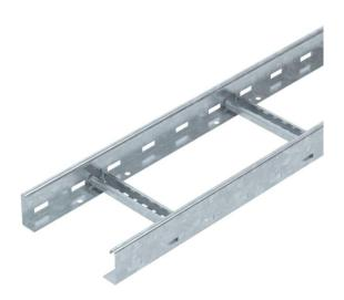
Cable ladder with a 60 mm side height with welded C30 profile rungs which are open in an upwards direction. Rolled side rail for reinforcement and as edge protection. Fastening to the bracket takes place using hold-down clamps, type LKS 40. The slot dimension of the rung is 16.5 mm and the appropriate clamp clip is type RS-H
