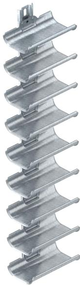
Cable support brackets for quick and easy routing of cables in areas where common cable support systems cannot be installed due to lack of space. The cable support brackets possess a large load-bearing surface as well as rounded outer edges to protect the cables. In accordance with DIN VDE 0298-300, a maximum support spacing of 0.8 m should not be exceeded.
