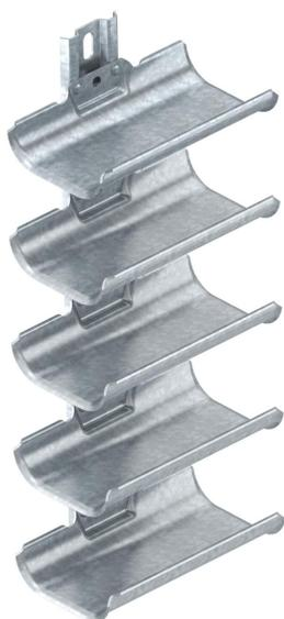
Cable support brackets for quick and easy routing of cables in areas where common cable support systems cannot be installed due to lack of space. The cable support brackets possess a large load-bearing surface as well as rounded outer edges to protect the cables. In accordance with DIN VDE 0298-300, a maximum support spacing of 0.8 m should not be exceeded.
