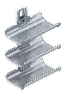
Cable support brackets for quick and easy routing of cables in areas where common cable support systems cannot be installed due to lack of space. The cable support brackets possess a large load-bearing surface as well as rounded outer edges to protect the cables.
