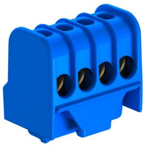
Neutral conductor connection terminal, brass, steel screws, electrogalvanised and transparently passivated, nominal cross-section 6  $\div$  16  $\text{mm}^2$ , nominal voltage 400 V, 1-pole, with terminal sockets, max. connectable conductors per terminal 4 x 16 mm<sup>2</sup>, 4 x 10 mm<sup>2</sup>, 8 x 6 mm<sup>2</sup> or 12 x 4 mm<sup>2</sup>.
