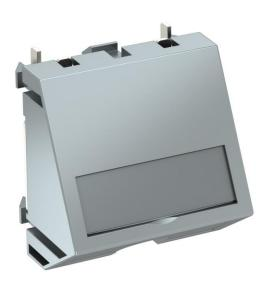
Two-part cable outlet with labelling panel, consisting of a cable support with strain relief and a cover. The strain relief is suited for cable cross-sections of 3 to 11 mm. The locking fastening is suitable for horizontal and vertical installation in the system environment.
