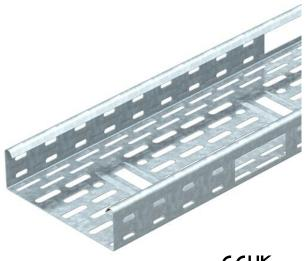
IKS 60 = installation cable tray system with 60 mm side height. Permeable cable tray system to VdS guideline 2092 with 30% hole surface for use under sprinkler systems.
