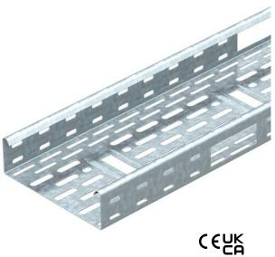
IKS 60 = installation cable tray system with 60 mm side height. Permeable cable tray system to VdS guideline 2092 with 30% hole surface for use under sprinkler systems.
