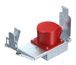
Device support of nominal size 3 with a CEE plug connection 16 A for installation in service outlets and cassettes of nominal sizes R7, 9 and R9. Device support with protective housing and strain relief. Required minimum installation depth: 190 mm when using a straight connector and 160 mm when an angled connector is used.
