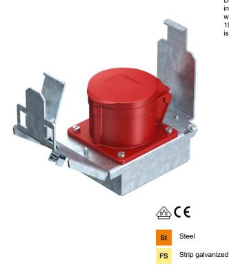
Device support of nominal size 2 with a CEE plug connection 16 A for installation in service outlets and cassettes of nominal size 2, 4, 6 and R7. Device support with protective housing and strain relief. Required minimum installation depth: 190 mm when using a straight connector and 160 mm when an angled connector is used.
