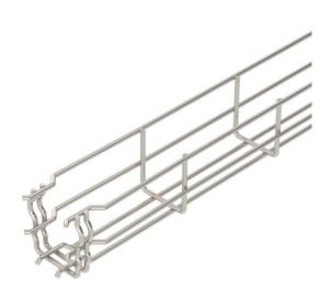
Mesh cable tray with shaped connector of side height 55 mm. No additional connection components are required for the mesh cable tray, it is simply interlocked. The grid width is 50 x 100 mm (exception: GRM 55/50 = 20 x  $^{\circ}$
