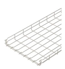
Mesh cable tray with shaped connector of side height 55 mm. No additional connection components are required for the mesh cable tray, it is simply interlocked. The grid width is 50 x 100 mm (exception: GRM 55/50 = 20 x 100 mm).
