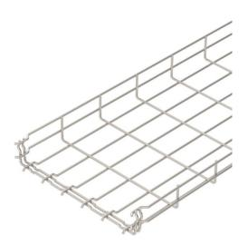
Mesh cable tray with shaped connector of side height 55 mm. No additional connection components are required for the mesh cable tray, it is simply interlocked. The grid width is  $50 \times 100 \text{ mm}$  (exception: GRM  $55/50 = 20 \times 100 \text{ mm}$ ).
