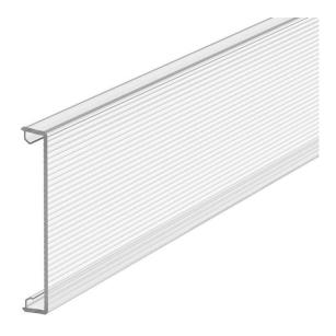
Trunking cover for closing Rapid 80 GK (PVC), GS (steel) and GA (aluminium) device installation trunking as well as ISS service poles with a 76.5 mm system opening. The GK-OTKKP cover is made from clear, transparent plastic and the inside is fluted (longitudinal) and is therefore suitable for integrating lighting in the trunking and service pole.
