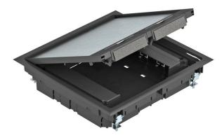
GES9 service outlet with a fixed construction height of 55 mm for use in installation trunking systems in dry rooms with dry-care floors in interior areas. With two installation housings for vertical mounting of Modul 45 devices and four strain reliefs. Two installation frames are required to mount Modul 45 devices.
