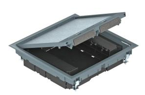
GES9 service outlet with a fixed construction height of 55 mm for use in installation trunking systems in dry rooms with dry-care floors in interior areas. With two installation housings for vertical mounting of Modul 45 devices and four strain reliefs. Two installation frames are required to mount Modul 45 devices.
