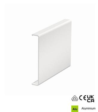
Aluminium cover, for closing Rapid GA device installation trunking and ISS service poles with a 76.5 mm system opening. The firm position of the cover and electrical contact to the lower part of the trunking and service pole is guaranteed thanks to type RKV3V locking brackets. There are 2 pre-mounted locking brackets included per delivery length (100 mm).
