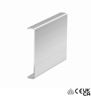
Aluminium cover, for closing Rapid GA device installation trunking and ISS service poles with a 76.5 mm system opening. The firm position of the cover and electrical contact to the lower part of the trunking and service pole is guaranteed thanks to type RKV3V locking brackets. There are 2 pre-mounted locking brackets included per delivery length (100 mm).
