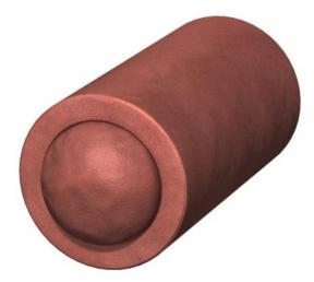
Pipe shell for cable insulation consisting of a one-part, hard pipe sleeve and two soft plugs with a 500 mm diameter. Protect the pipe sleeves and plugs against water in order to guarantee safe foaming in case of fire. Application in interior areas.
