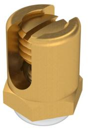
Earthing terminal for fastening the equipotential bonding wire to the cable support system. M12 threaded pin with slot. Suitable for conductor cross sections of 4-50 mm<sup>2</sup>. With serrated washer and lenshead screw.
