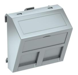
Data technology support with slanting outlet and locking slider to accept two data technology connection modules with RJ45 socket. The locking fastening is suitable for horizontal and vertical installation in the system environment. Type EP has a special module seat and is designed for indirect fastening of the data connection modules in the mounting opening.
