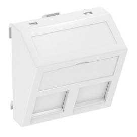
Data technology support with slanting outlet and locking slider to accept two data technology connection modules with RJ45 socket. The locking fastening is suitable for horizontal and vertical installation in the system environment. Type C has a mounting opening of 19.30 x 14.80 mm and is designed for direct fastening of the data connection modules in the mounting opening.
