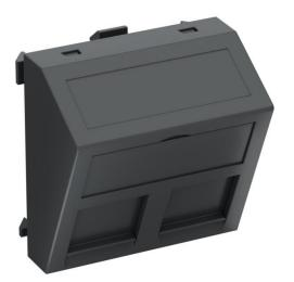
Data technology support with slanting outlet and locking slider to accept two data technology connection modules with RJ45 socket. The locking fastening is suitable for horizontal and vertical installation in the system environment. Type B has a mounting opening of 19.35/21.55 x 14.85 mm and is designed for direct fastening of the data connection modules in the mounting opening. The type B data technology support is suitable for accepting the following data
