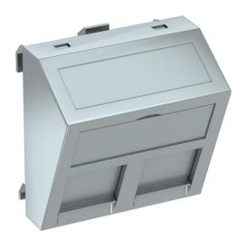
Data technology support with slanting outlet and locking slider to accept two data technology connection modules with RJ45 socket. The locking fastening is suitable for horizontal and vertical installation in the system environment. Type B has a mounting opening of  $19.35/21.55 \times 14.85$  mm and is designed for direct fastening of the data connection modules in the mounting opening.
