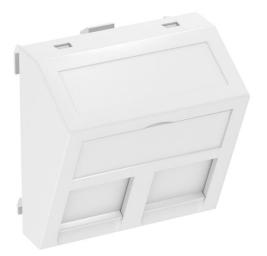
Data technology support with slanting outlet and locking slider to accept two data technology connection modules with RJ45 socket. The locking fastening is suitable for horizontal and vertical installation in the system environment. Type A has a mounting opening of 20.10 x 14.80 mm and is designed for direct fastening of the data connection modules in the mounting opening.
